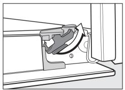
■ To release the locking clamps on the hinges turn them upwards as far as they will go until they are at an angle. See illustration.
